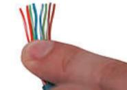
**7-** Carefully insert the flattened, arranged wires into the connector, pushing through until the wire ends emerge from the pins.
